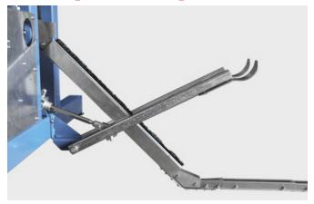
Pnuematically operated strap guide arms for precise positioning of the strap on the paper roll
