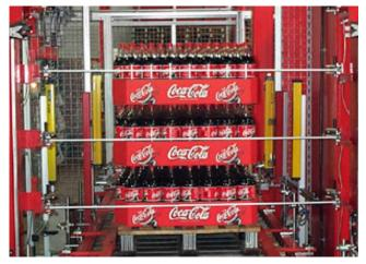
Strap is applied by the movement of the product passing through the machine. Strap cycle time is six seconds.
