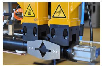
Simple sealing head with few moving parts and low maintenance operation.
