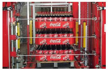
Strap is applied by the movement of the product passing through the machine. Strap cycle time is six seconds.
