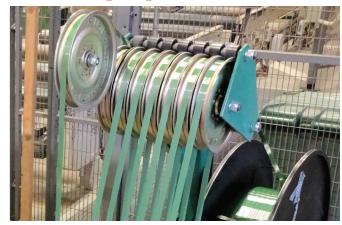
The PSD-119J jumbo dispenser is an all mechanical strap accumulator design for reliability and performance when paired with Z-20 head modules.
