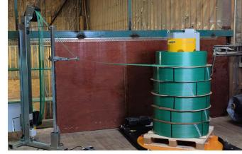
Increase uptime with the optional OR-A600J multi-coil strap dispenser. Load up to six coils of strap on the rotating turntable.
