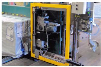
The easily accessible head carriage allows easy service work when needed. Signode model Z-20 modular head technology improves performance and speed.
