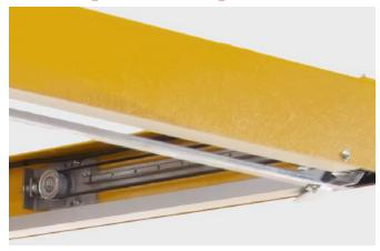
Electrical driven strap guide system for exact strap placement positioning.
