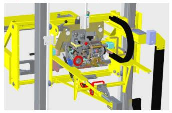
The easily accessible carriage swivels 90° for accessibility to the strapping head for service and maintenance.
