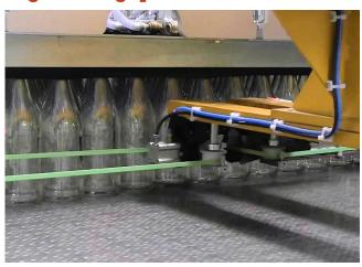
Strap is applied by the movement of the product passing through the machine. Strap cycle time is six seconds.
