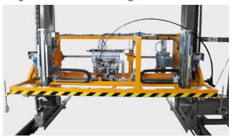
Fast variable speed drive motor with three-fold safety level on lifting chains. Lightweight space-frame model for high speed productivity. Optional heavy duty compression platen and top edge-protection applicator available.
