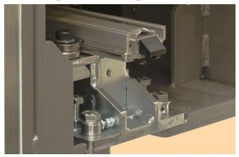
Low height bayonet or special protected bayonet for flexibility. Adjustable speed of bayonet for higher customisation and higher throughputs. Full-length strap-flaps on bayonet for increased reliability.
