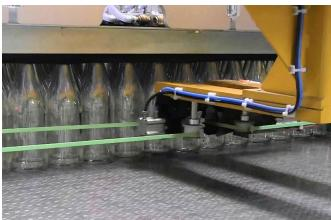
Strap is applied by the movement of the product passing through the machine. Strap cycle time is six seconds.
