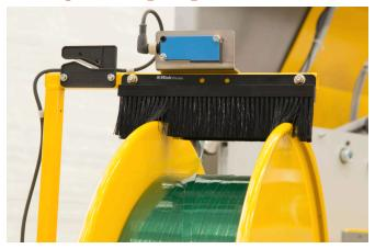
Intelligent dispenser with auto strap feed-up and re-feed from dispenser into sealer for medium and light-duty MHC heads.
