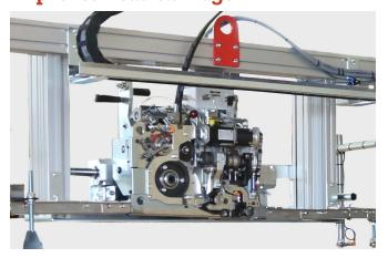
Fast variable speed drive motor with three-fold safety level on lifting chains. Lightweight space-frame model for high speed productivity. Optional heavy duty compression platen and top edge-protection applicator available.
