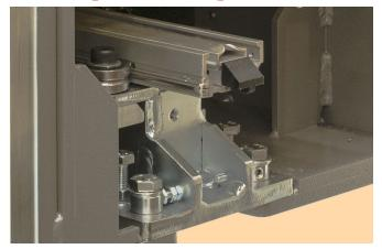
Low height bayonet or special protected bayonet for flexibility. Adjustable speed of bayonet for higher customisation and higher throughputs. Full-length strap-flaps on bayonet for increased reliability.
