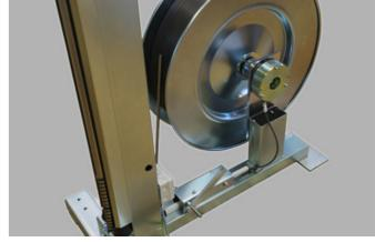
Equipped with strap end pre-warning. Coil changes can be prepared to maximize productivity and machine up time.
