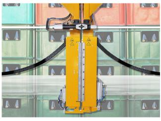
Strap and Film Band is applied by the movement of the product passing through the machine. Cycle time is six seconds.
