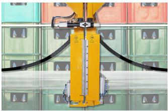
Strap and Film Band is applied by the movement of the product passing through the machine. Cycle time is six seconds.
