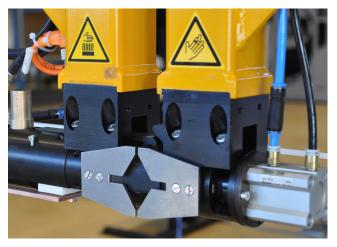
Simple sealing head with few moving parts and low maintenance operation.
