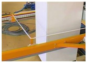
Strap is applied by the movement of the extension arm finger guides wrapping the strap around the product. Very accurate postioning of the strap placement.
