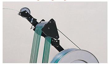
Standard dispenser for medium and heavy duty applications. Jumbo dispenser station option for maximum machine uptime.
