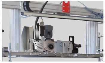
Fast variable speed drive motor with three-fold safety level on lifting chains. Lightweight space-frame model for high speed productivity. Optional heavy duty compression platen and top edge-protection applicator available.
