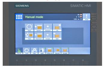
An icon driven control panel that provides step by step prompts for easy and intuitive set up, with minimal language used, for simple control of all functions from a single panel.
